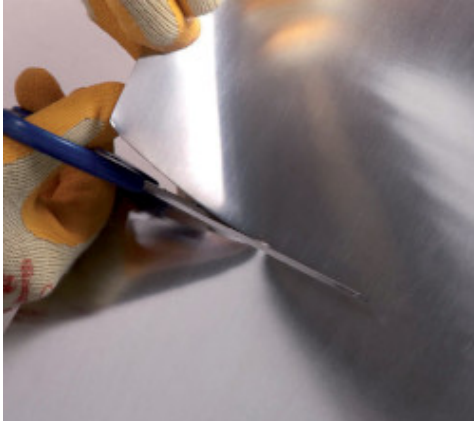
Unwinding and plate cutting
